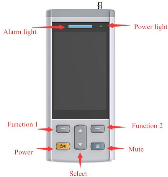
Fig. 1-1 buttons and indicator light
